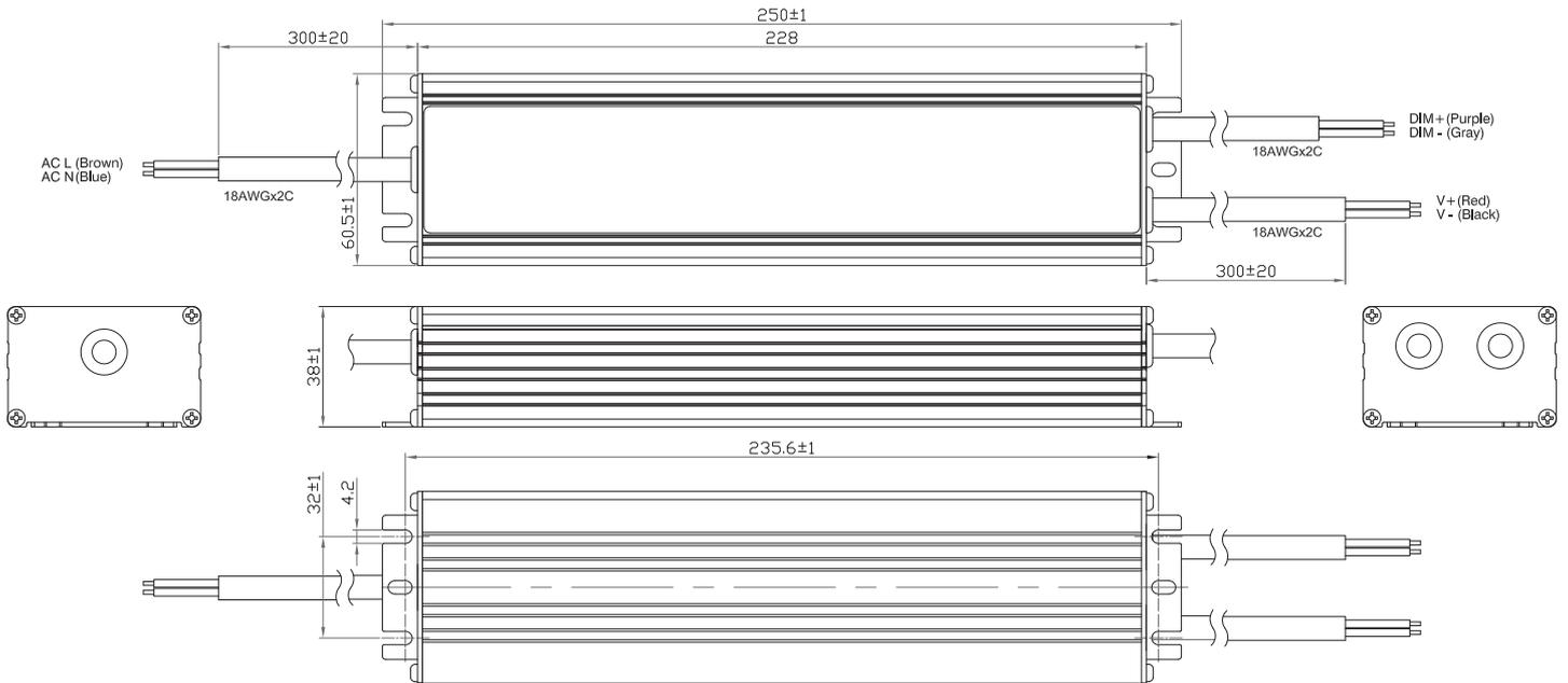
**Blank Type(Non-dimming): SAE-150-(700/1400/2100)**
